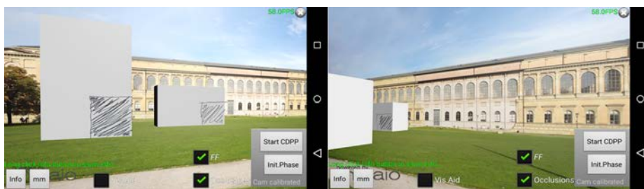
Fig. 10. Due to the image feature tracking, it is possible to walk through the scenario. As long as the tracked element is in sight, the object are displayed on real position.
