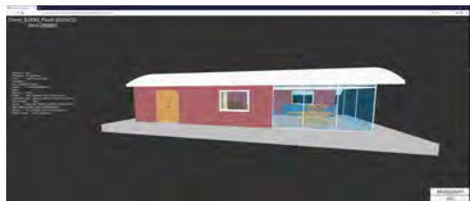
Figure 4. WebGL version of the tool. The user can query BIM information from the elements and navigate around the model. It is also possible to join a session hosted on a PC version of the tool and collaborate. VR via Web is supported.
